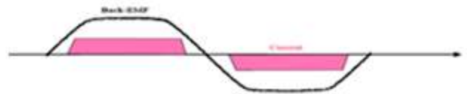
Fig. 2.1. The phase current is in phase with the back EMF in brushless dc motor.
